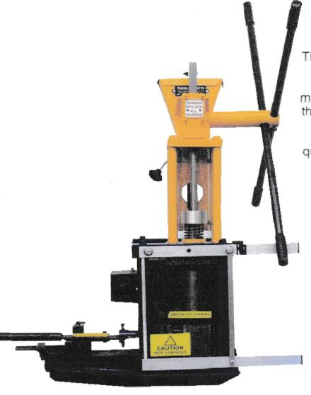
The TP2 hand operated machine still offers all the same advantages as the TP1 with the exception of the Air operated injection unit. The TP2 injects via the manually operated star wheel through a rack & pinion gearbox. This machine will produce the same high quality mouldings as the TP1
